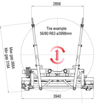
Cradle stroke: 450mm (vertical) Cradle tilting capacities: Forwards/backwards approx.  $\pm 10^{\circ}$ Sideways approx.  $\pm 10^{\circ}$
