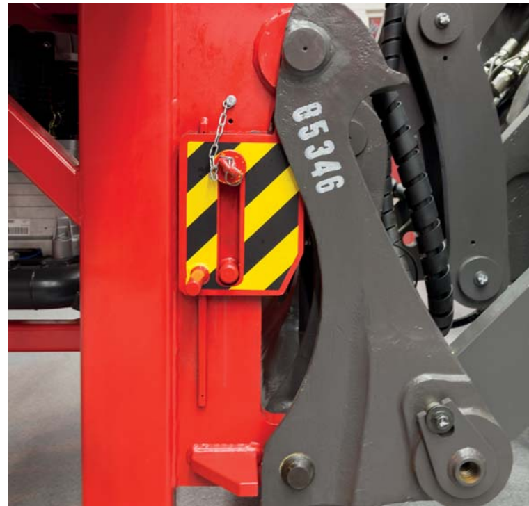
A patented safety lock ensures that the MEWP is impossible to dislodge from the attachment bracket.
