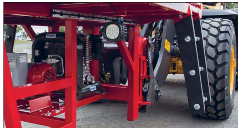
BK008 comes with a range of optional equipment such as; a two speed concrete pump, power generator, compressor, etc. which is mounted in a protected position on the under carriage.
