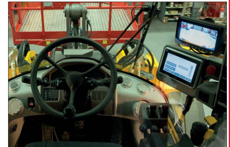
Both the carrier and the MEWP can be controlled from inside the driver's cab...
