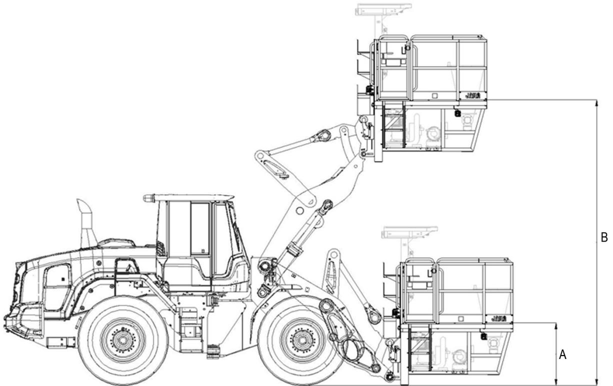
Mobile elevating working platform (MEWP) BK008/SL009 is together with Jama-modified versions Volvo wheel loader L70, L90 and L120 F \*, certified and approved for lifting persons. The platform can be operated either from the cabin or from the platform.
